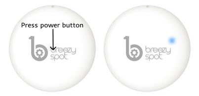
2. Using a Breezy Smart Controller that has been configured to the site, tap the Breezy Spot button on the devices Screen.
